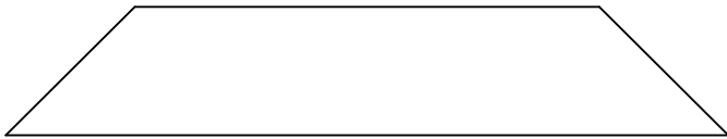
Step One: Cut miter on ends
