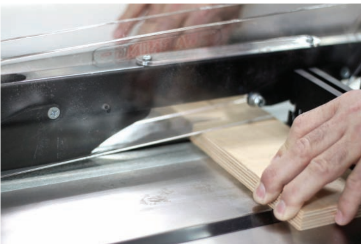
5 Keep your hands out of path of the saw blade.
