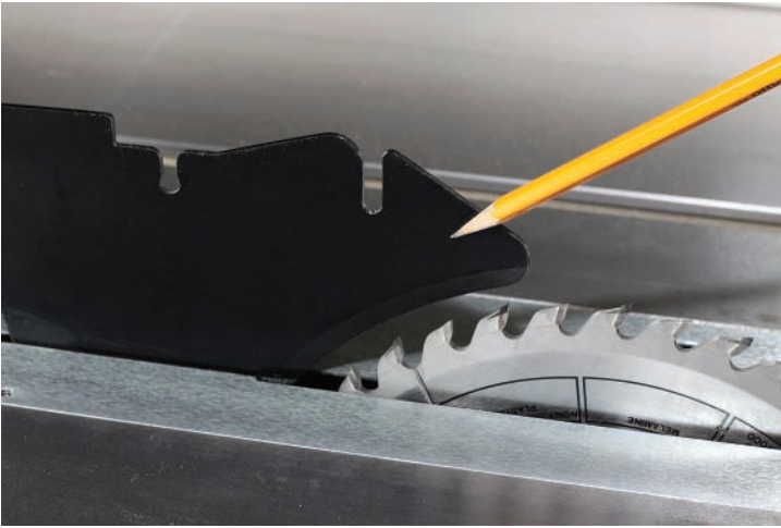
13 Use a splitter or riving knife to prevent kickback.
