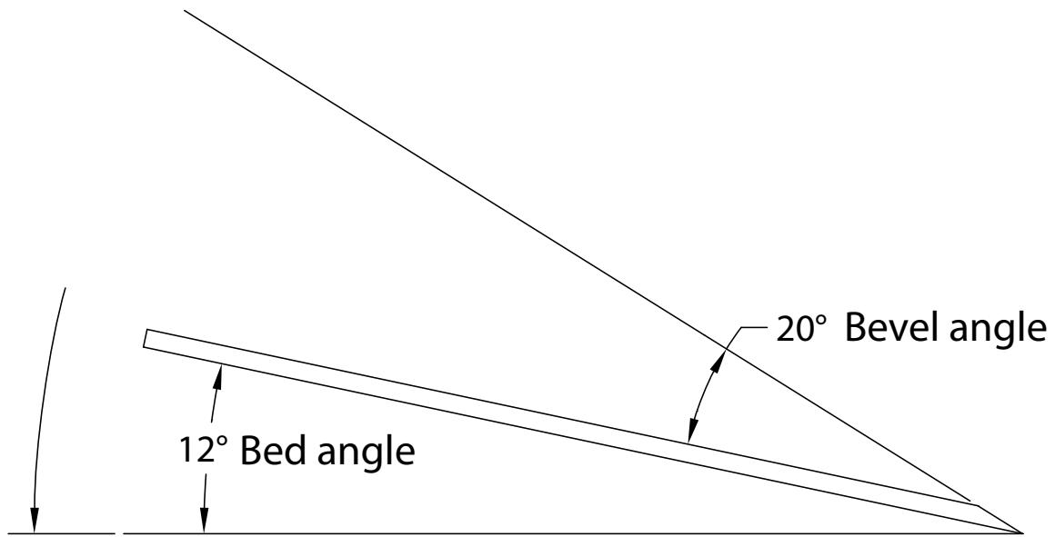
Low angle block plane cutting geometry
